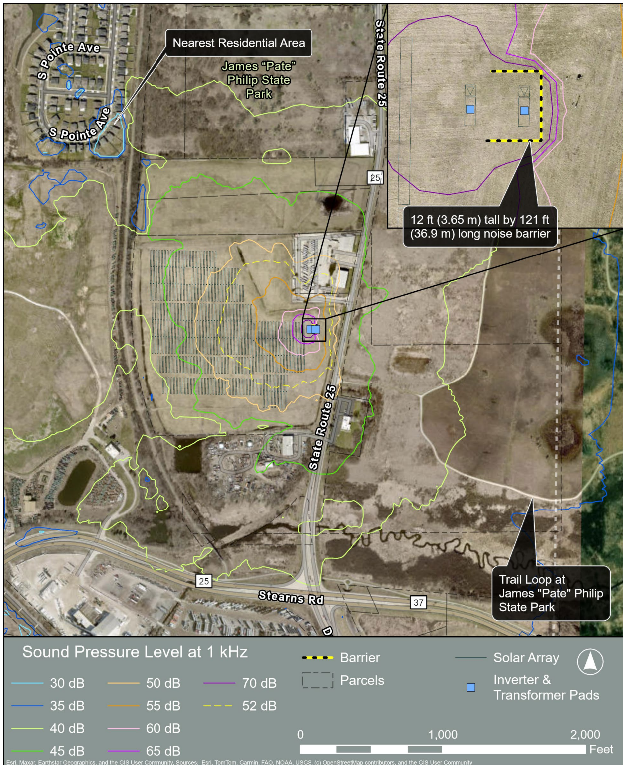
Figure 3: Mitigated Model Results Map for the 1 kHz Octave Band Showing a Potential Noise Barrier
